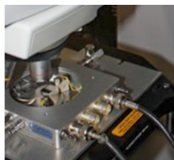
Photograph of the Linkam HFS600E-PB4 probe system in the lab at RMIT, where it is used to apply an oscillating electric field during Surface Enhanced Raman Scattering.
